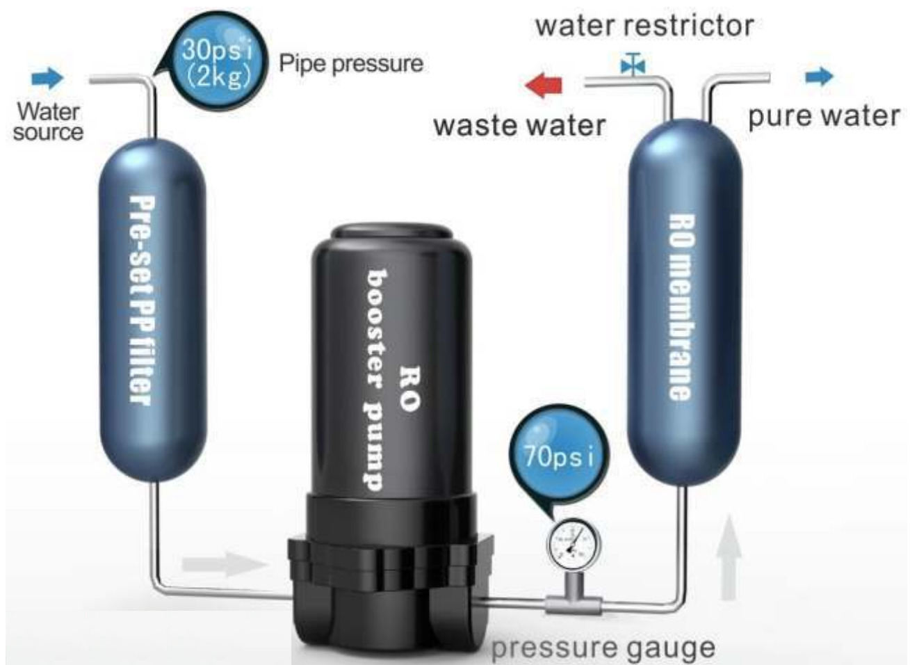
Diagram of how Diaphragm Booster Pump works
